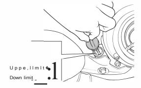
**Using the recommended type of oil** SAE 10W-30(SIGMA) for 4-stroke engines or its substitute HQB-10 should be used.
