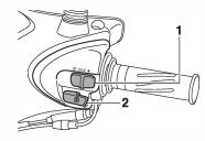
Run/ Stop switch (1) Slide the switch to the circle to start the engine slide the switch to the circle sith and X to turn off the engine
